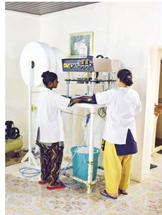
Each of the AAKAR Innovations factories employs 15 women in production. In this picture, two women are making sanitary pads using the semi-automatic pad sealing machine in the Adgaon Unit.
