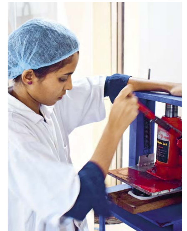
AAKAR Innovations customised four machines and two specialised tools for each mini factory. Here, a worker is cutting air-laid paper using the hydraulic air-laid cutting machine in the Adgaon unit.
